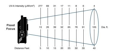
Radiometric data for MHL450 Lamp
